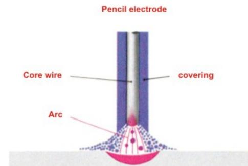
Figure 3: Principle of manual arc welding
