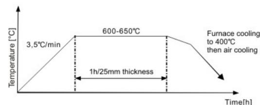
According to each 25mm effective thickness of the workpiece hold one hour to account the temperature holding time.
