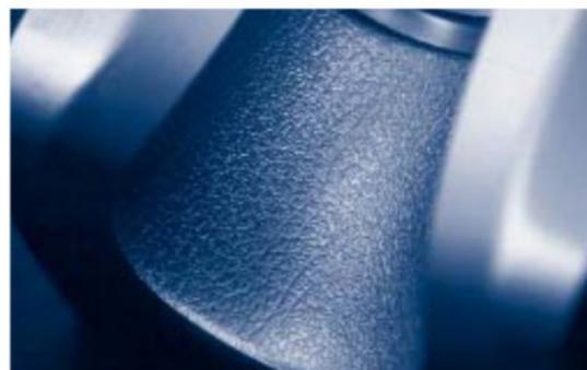
Leather structure grain on the cavity side of a plastic injection mould
