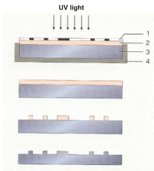
Principle of photo-etching
