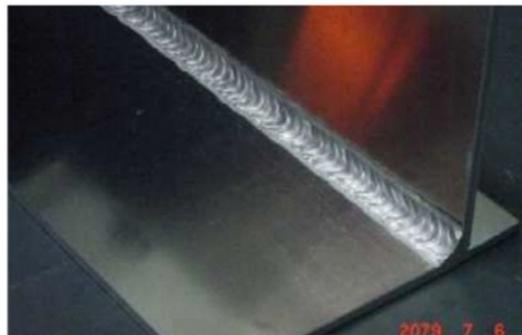
Figure 2: MIG fillet weld
