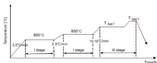
High pressure N<sub>2</sub> quenching ≥ 9 bar (min 28°C/min) cooling to 500°C, reduce pressure appropriate
