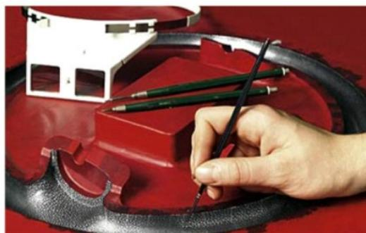
Preparing the relevant mould surface with a film negative before etchingA
